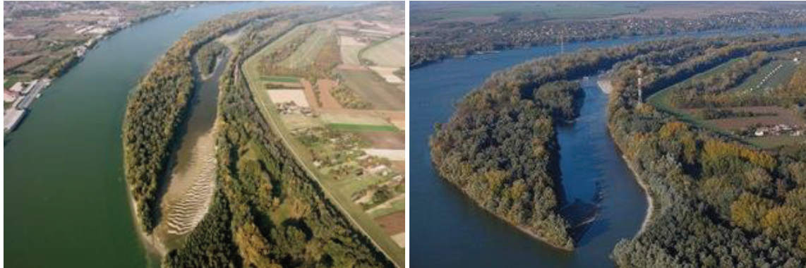
Figure 2: Restoration of Szabadság-island in the Danube River. Example for reconnecting side branches. reach scale measures. (source: https://wwf.hu/hireink/vizeselohelyek/ujra-vizi-paradicsom-a-szabadsag-sziget/ )
